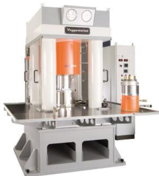
Large-volume press for ND synthesis at MPIP.
